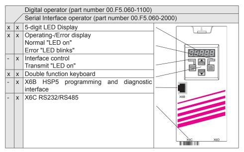
Do not connect a PC to the operator interface connector on the COMBIVERT R6 unit! Damage to the PC may result. Direct connection, PC to the COMBIVERT R6 is only possible with a special cable HSP5 cable (part number 00.F5.0C0-0010) or USB Converter Cable (part number 00.58.060-0020)
