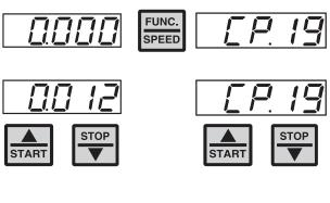
Generally, changes to parameter values are immediately accepted and stored non-volatile. However, with some parameters, due to their functionality, the adjusted value is not accepted immediately. With these parameters (see parameter overview) the adjusted value is accepted and stored non-volatile by pressing ENTER.
