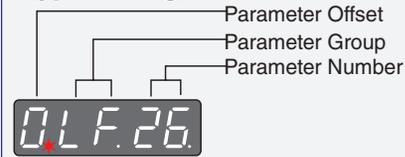
Press **Enter** to move the blinking dot laterally. The number/group to the left of the blinking dot is the active (changeable) part of the parameter
