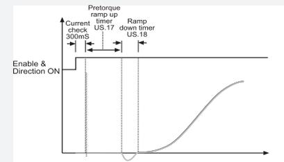
When adjusted properly, the brake should pick, the motor holds the load for a short period (about 1/4 second) and then the acceleration begins.
