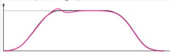
High values (10,000) can cause high frequency oscillation resulting in vibration or a buzzing sound in the motor.
