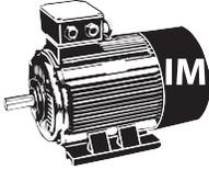
For an **Induction Motor** you may **NOT** enter the motor-synchronous speed (e.g. 1200 rpm for a 6 pole, 60Hz motor) Rated Motor Speed = Synchronous Speed - Slip Speed. Ask the motor manufacturer for the motor rated speed.
