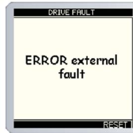
The LCD operator incorporates a real-time clock. This enables faults and special events to be recorded with a time-stamp in the Diagnostics Screen Log. To set the date and time, refer to Section 4.10. With the SD Card keypad operator hardware version, the clock stops when the keypad is not powered on. With Serial/CAN keypad operator hardware version, the clock continues even when not powered on.
