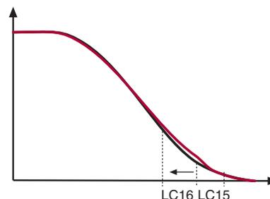
Speed for Min. Integral Offset Deceleration too low for gearless - Speed begins to lag during deceleration but then recovers in the final approach.
