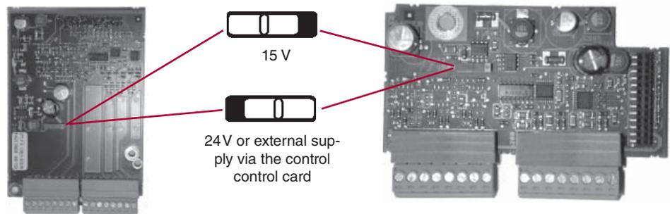
The maximum load capacity is dependant on the selected voltage supply.
