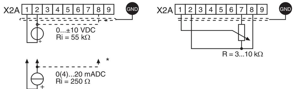
Connect unused analog inputs to common to eliminate noise signals!
