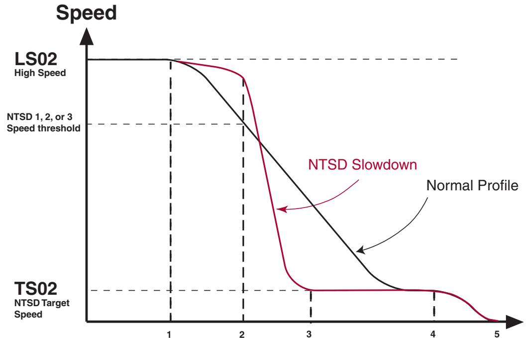
The diagram above and corresponding sequence (1-5) descriptions below show an example of a normal run (A) and a run in which the NTS is initiated (B).
