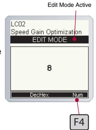
An example of using the NUM function to change a parameter is shown below:
