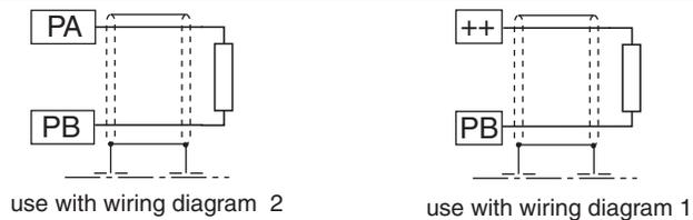
**Braking resistor with lineside overtemperature cutoff**
