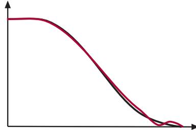
Integral Offset Deceleration Too Low (500) - Speed lags command during final transition into leveling speed. Speed may appear to spot or stop briefly just before stop; may undershoot floor.
