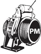
For PM Synchronous Motors, the relationship between the rated motor speed, rated motor frequency and the number of motor poles **MUST NOT** include any slip.
