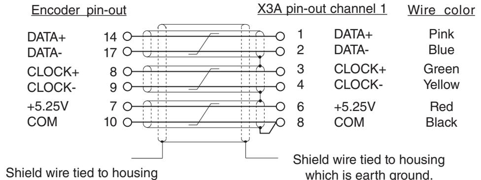
**Note: Inner pair shields are tied to 0V (com), not earth ground!**
