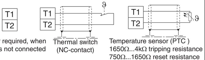
**Connection of braking resistor (Braking circuit installed as standard in housing sizes E,G,H, R and U.)**
