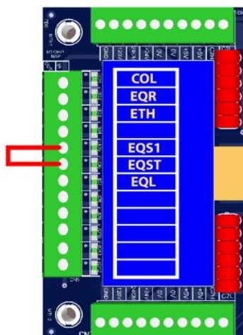
Figure 2: Typical I/O Expansion Board Earthquake I/O Board (if used)
