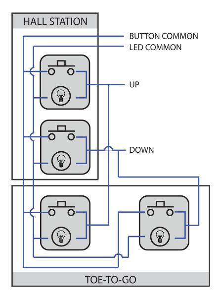
Screw terminals in parallel with hall station or car operating panel pushbuttons.
