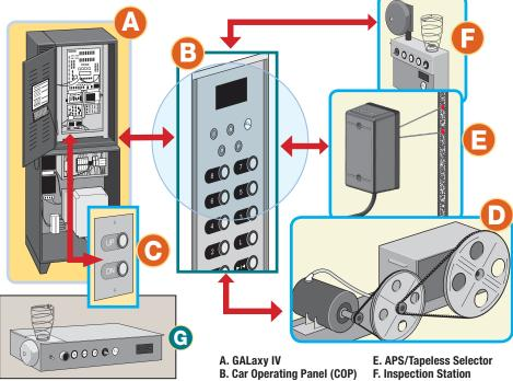
\*NOTE: Controller can be configured for traveling cable connections to Car Top Box or Car Operating Panel
