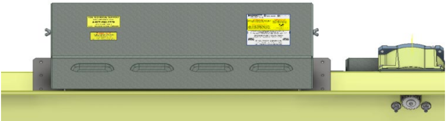
Figure3: MONXT drive box assembly with Support angles.
