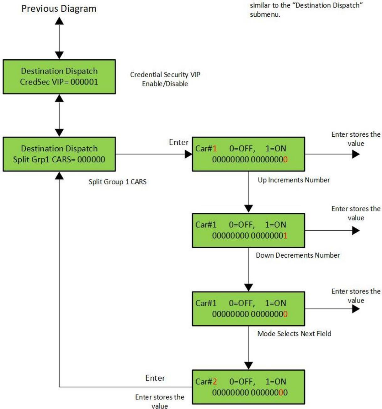
**Figure 5-8-4: The Destination Dispatch Submenu of the LCD Interface**
