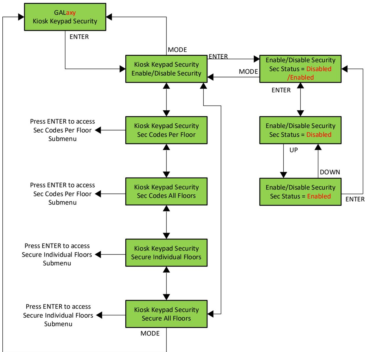
**Figure 5-23: LCD Interface Main Menu – Kiosk Keypad Security Menu**
