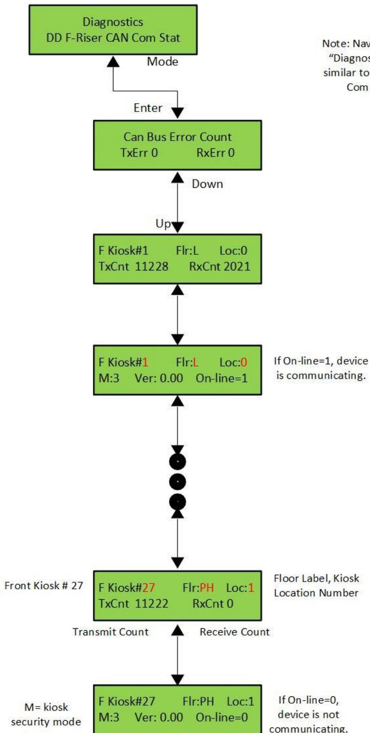
**Figure 5-16: LCD Interface Main Menu – DD F-Riser CAN Comm Status Submenu**
