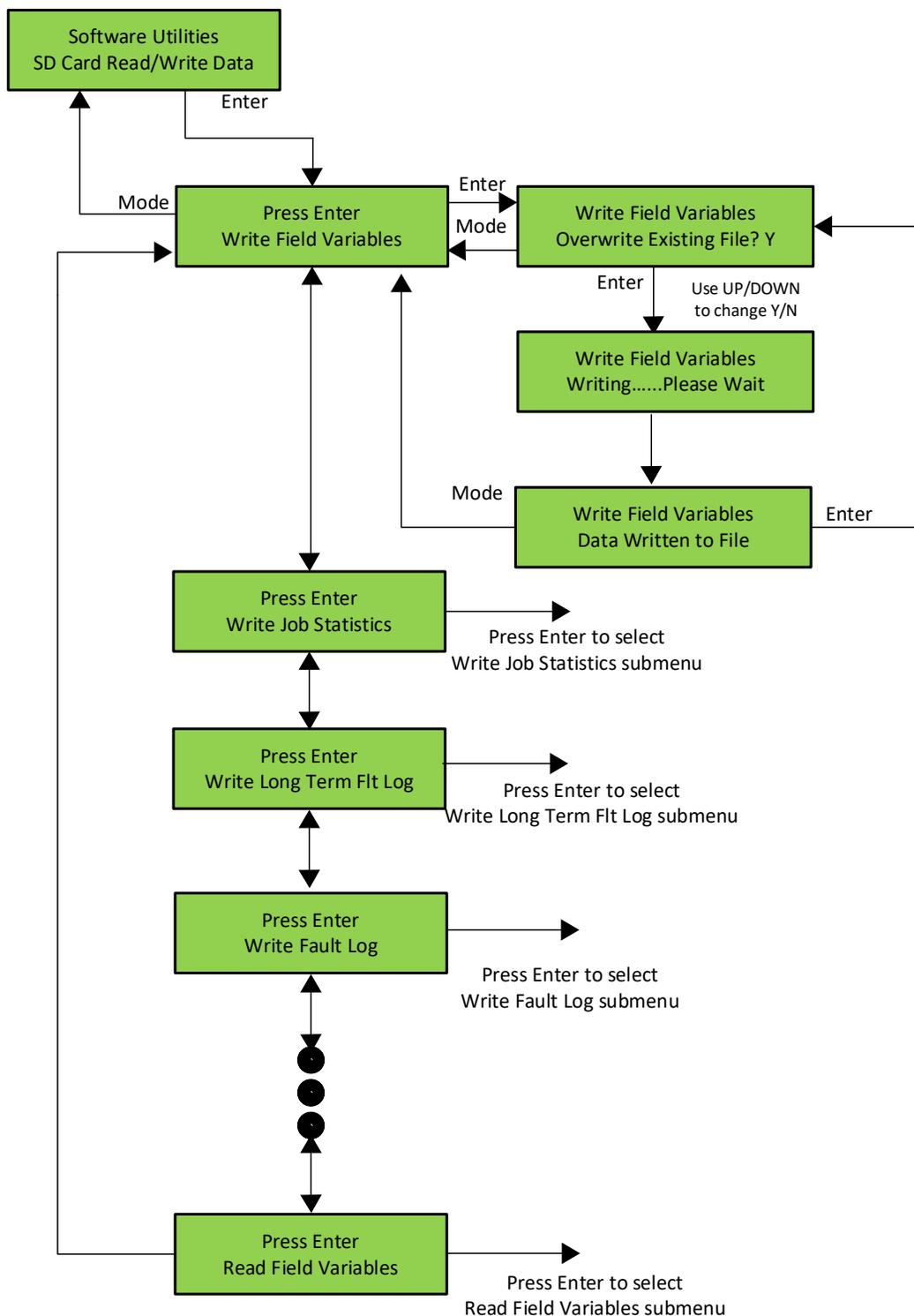
**Figure 5-20: LCD Interface Main Menu – SD Card Read / Write Data Submenu**
