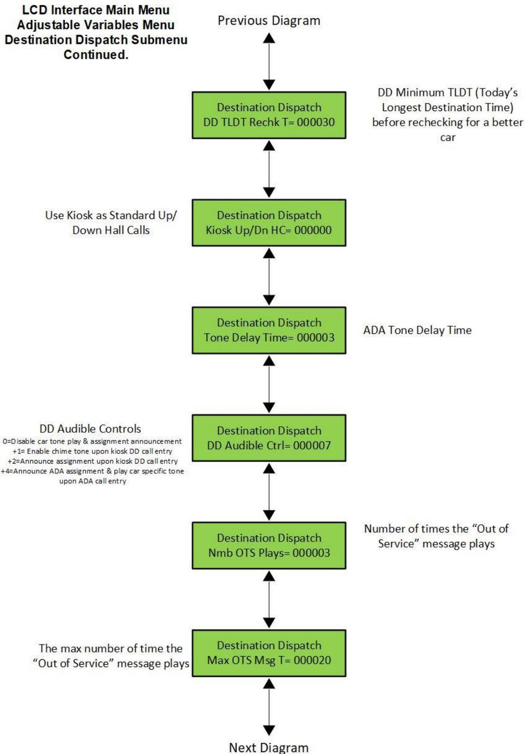
Figure 5-8-3: The Destination Dispatch Submenu of the LCD Interface
