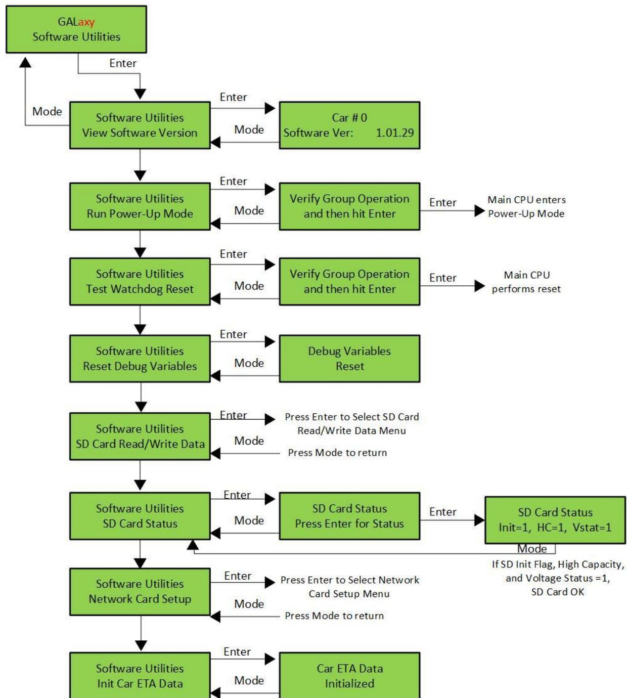
**Figure 5-17: LCD Interface Main Menu – Software Utilities**
