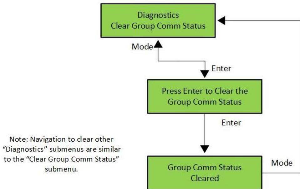
**Figure 5-15: LCD Interface Main Menu – Clear Group Comm Status Submenu**
