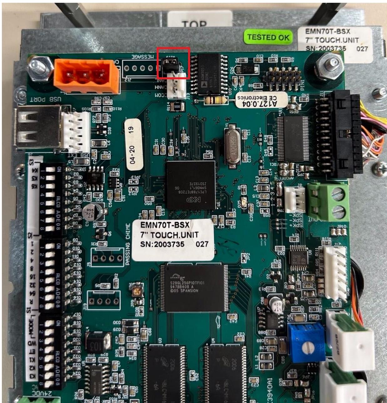
Figure 3-5: CAN Bus Jumper on C.E. Electronics Kiosk
