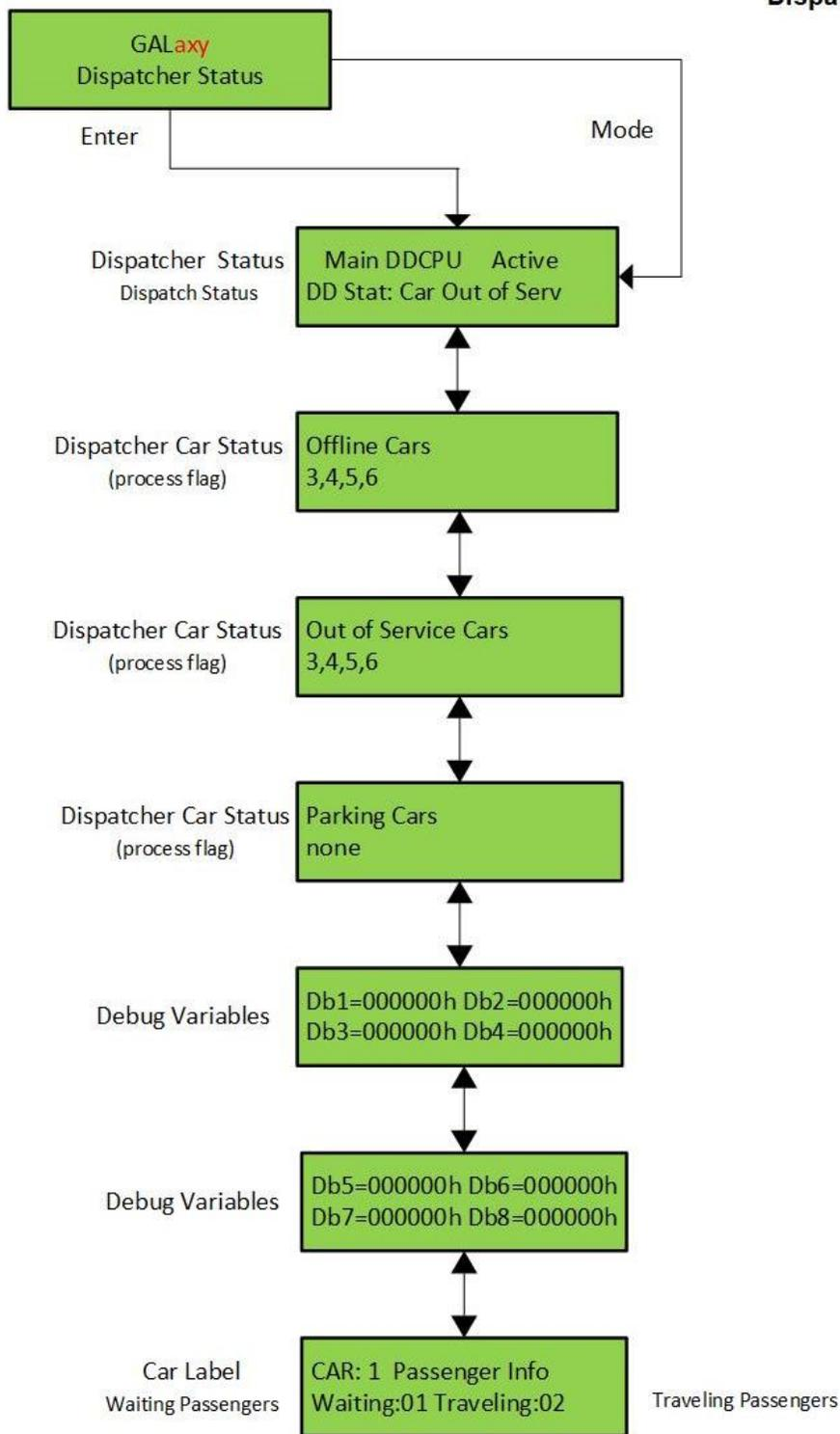
**Figure 5-2: The Dispatcher Status Menu of the LCD Interface**
