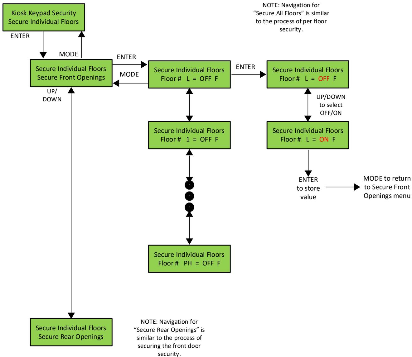
**Figure 5-25: LCD Interface Main Menu – Secure Individual Floors Submenu**
