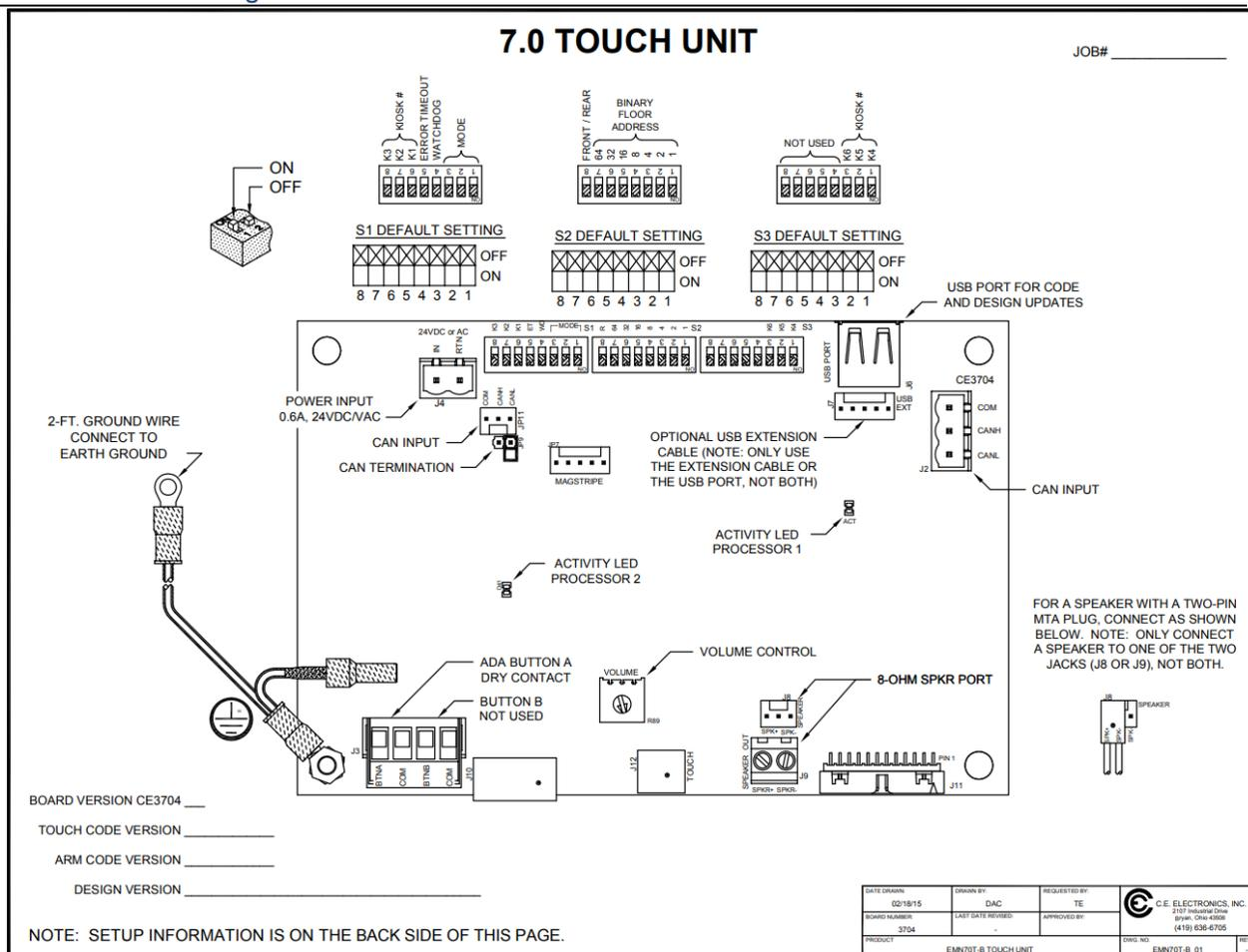
Figure 2-4: C.E. Electronics Sample Kiosk Wiring Diagram
