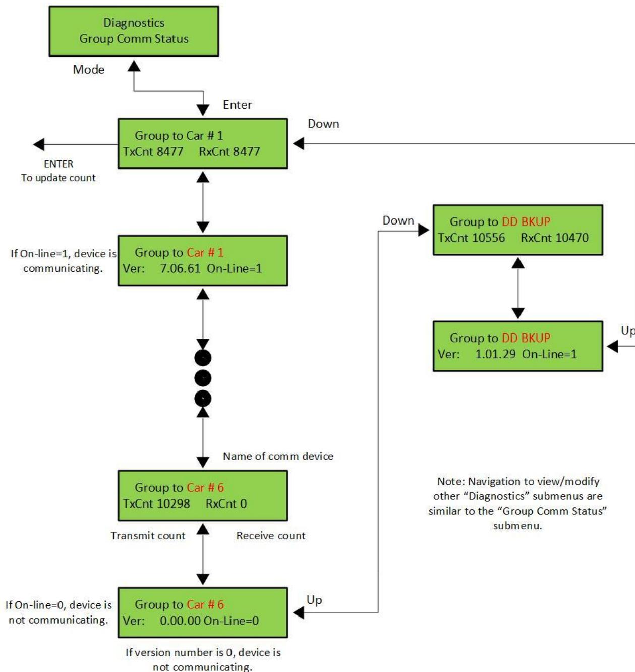
**Figure 5-14: LCD Interface Main Menu – Group Comm Status Submenu**
