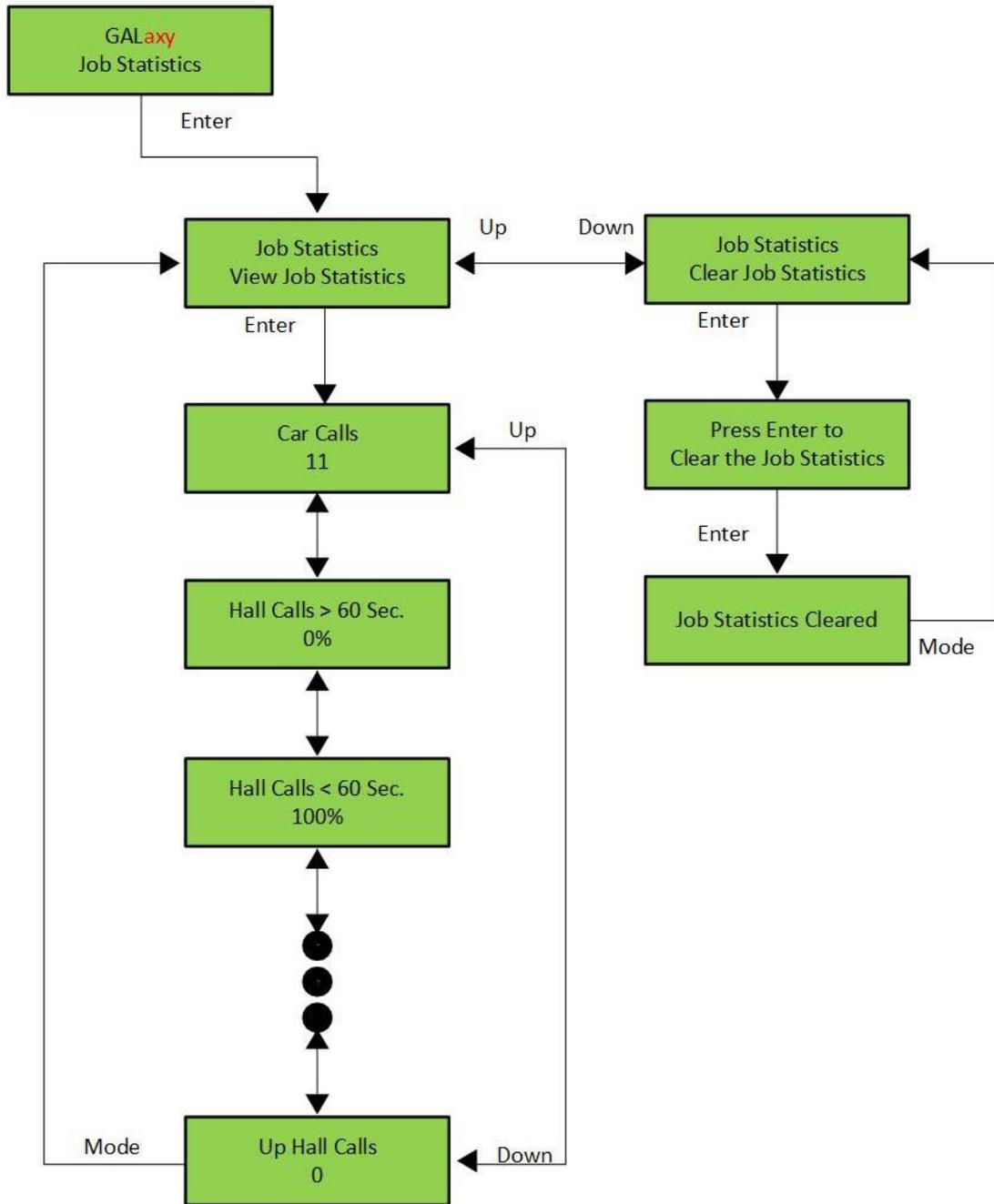
**Figure 5-6: The Job Statistics Menu of the LCD Interface**
