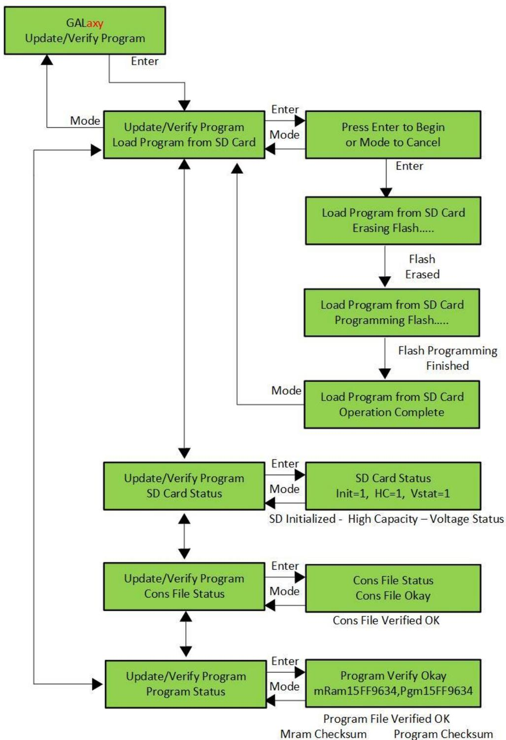
**Figure 5-19: LCD Interface Main Menu – Update / Verify Program Submenu**
