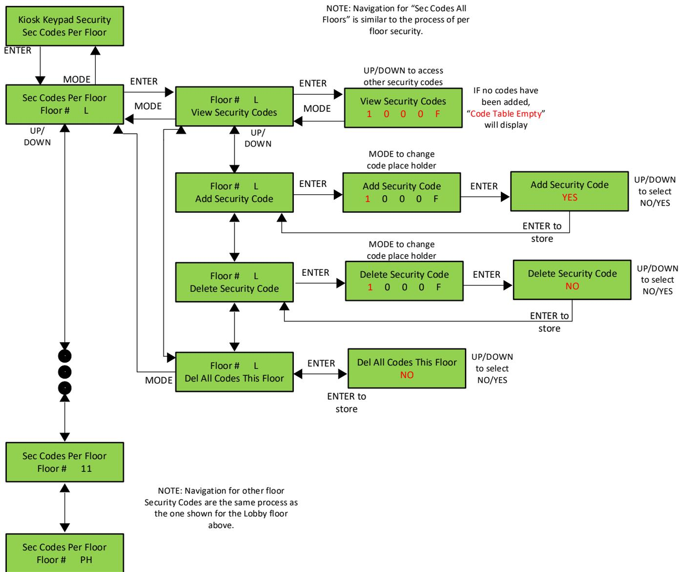
**Figure 5-24: LCD Interface Main Menu – Sec Codes Per Floor Submenu**
