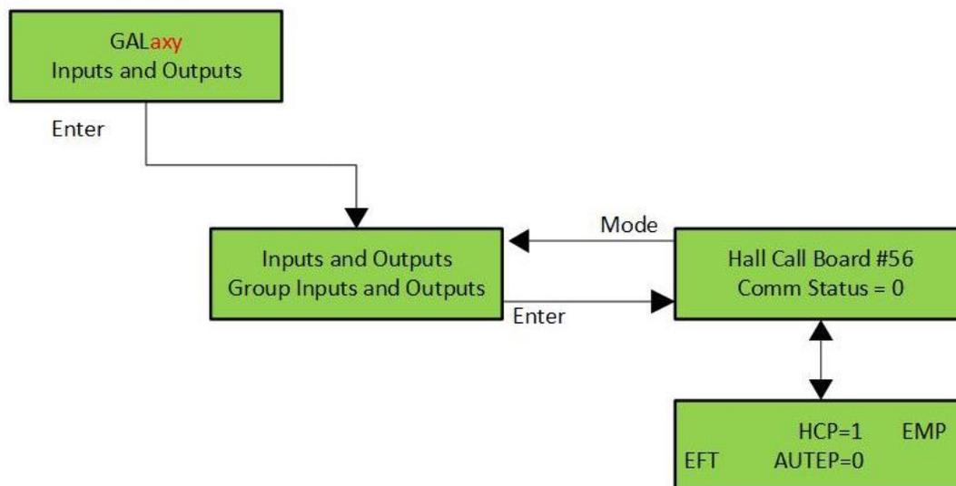
Figure 5-5: The Inputs and Outputs Menu of the LCD Interface
