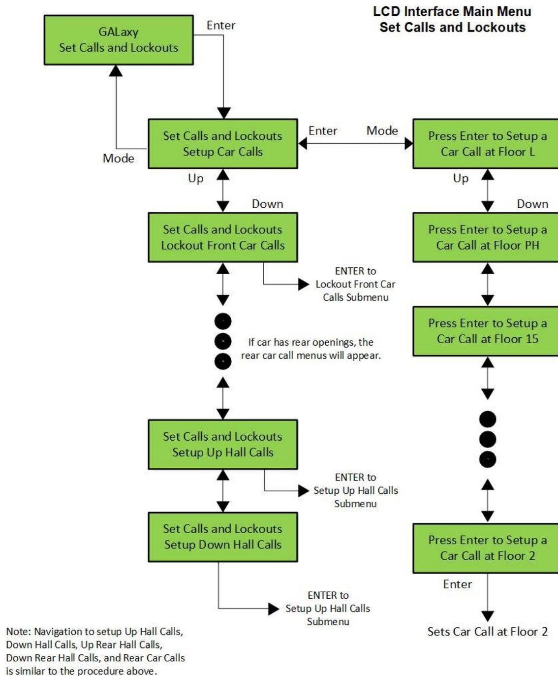
**Figure 5-3: The Set Calls and Lockout Menu of the LCD Interface**
