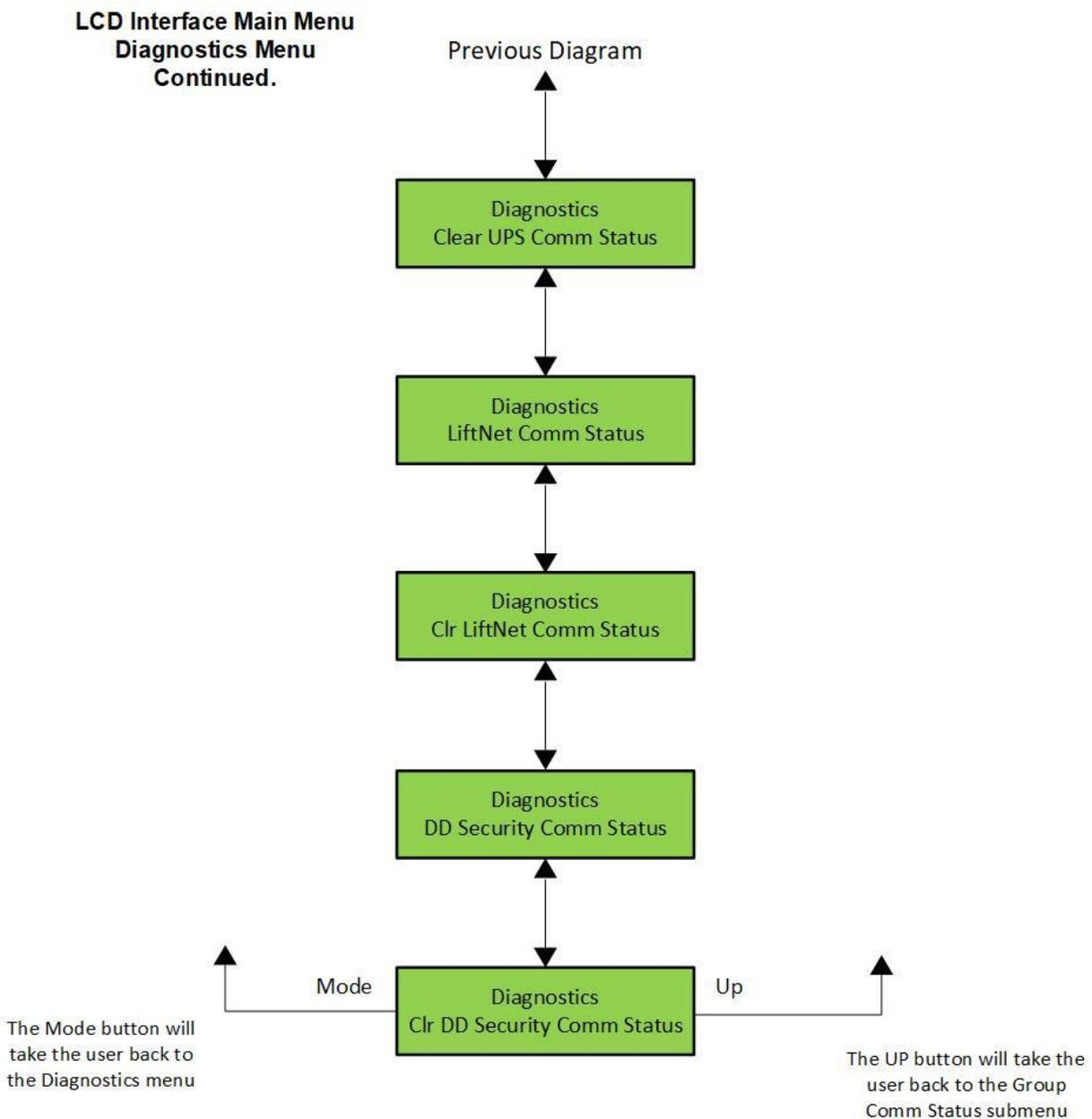
**Figure 5-5-3: LCD Interface Main Menu - Diagnostics**
