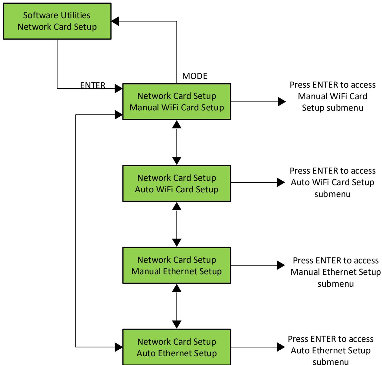
**Figure 5-21: LCD Interface Main Menu – Network Card Setup Submenu**
