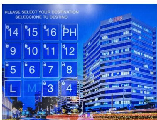
**Figure 8-2: Credential Security Enabled, With Lobby Floor Accessible**
