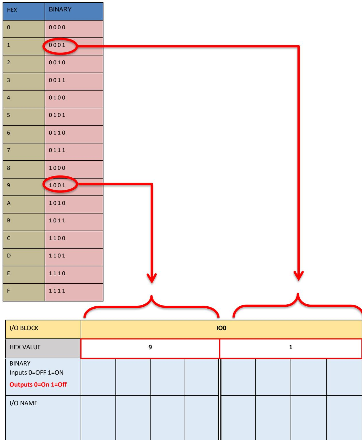
Place the Binary value for D (1101) in the first four bit locations and then place the binary value for 1 (0001) in the last four bit locations. The 1's show which inputs are on.
