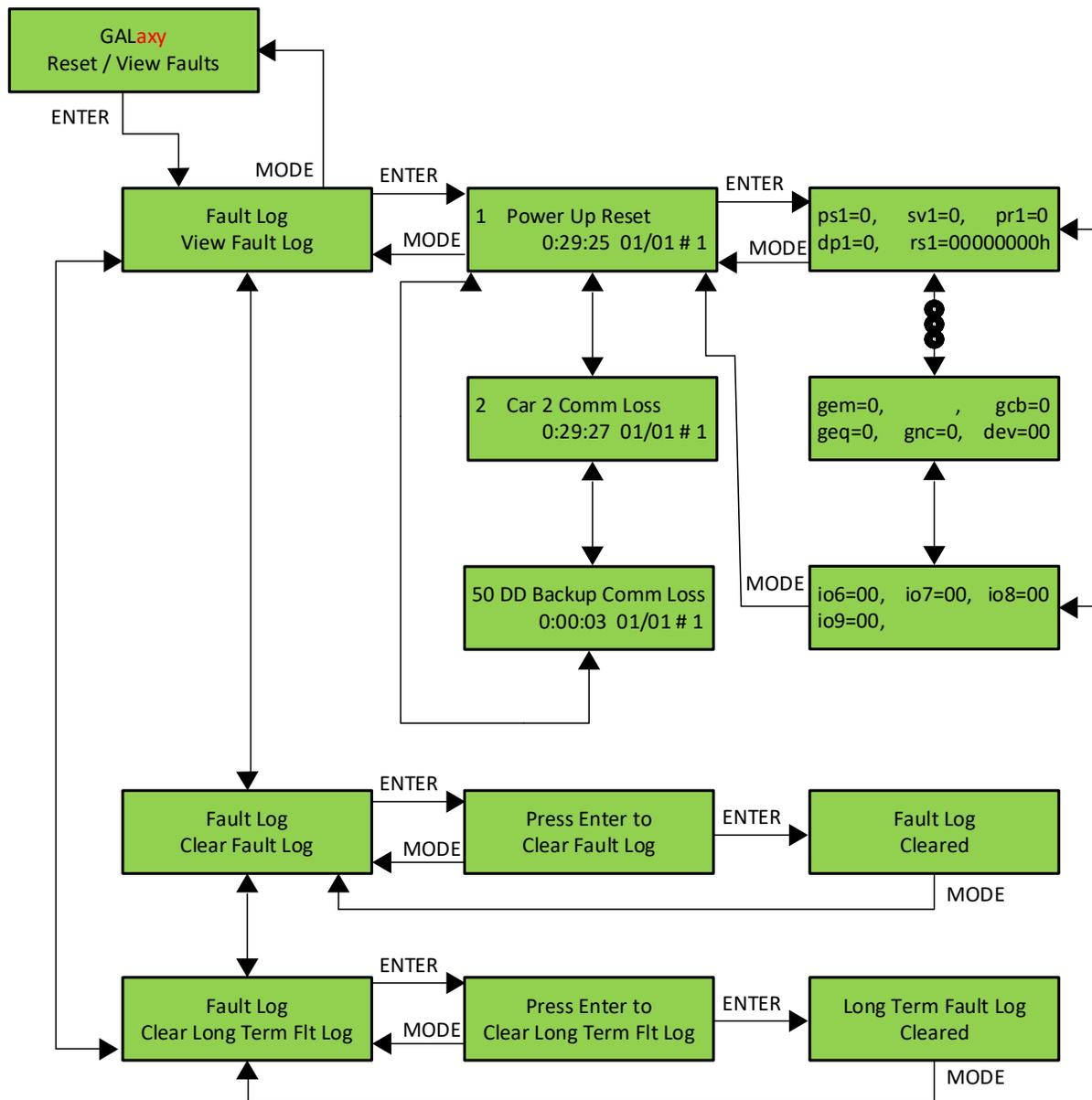
Figure 5-26: LCD Interface Main Menu – Fault Log Menu
