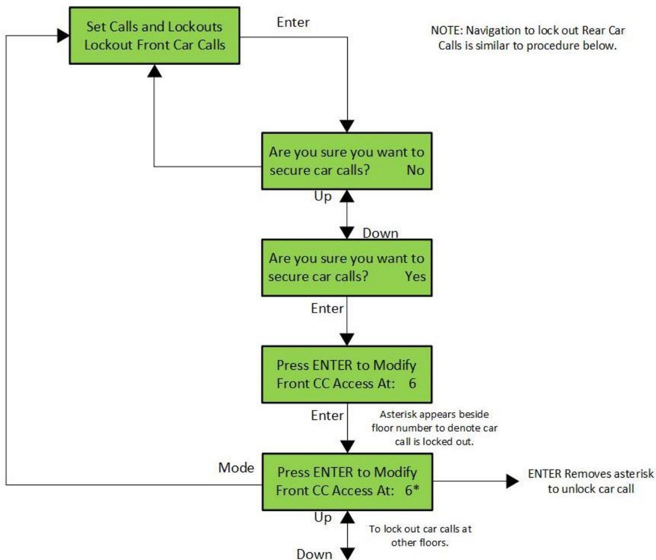
**Figure 5-4: The Front Car Call Lockout Submenu of the LCD Interface**
