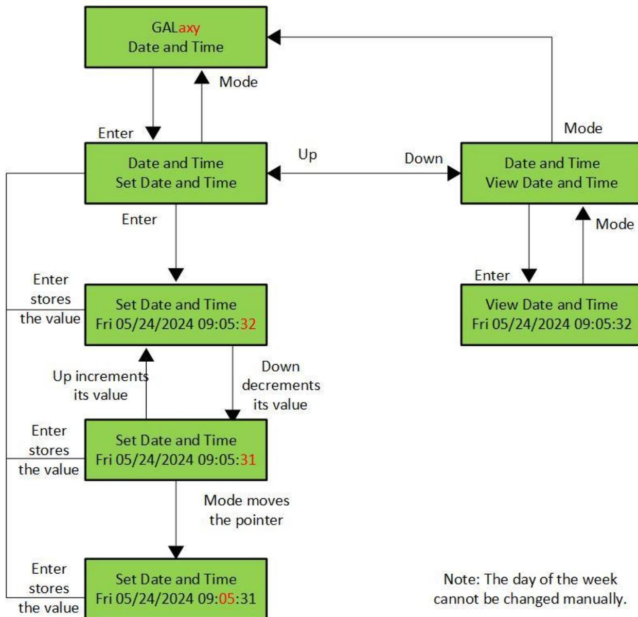
Figure 5-2: LCD Interface Main Menu – Date & Time
