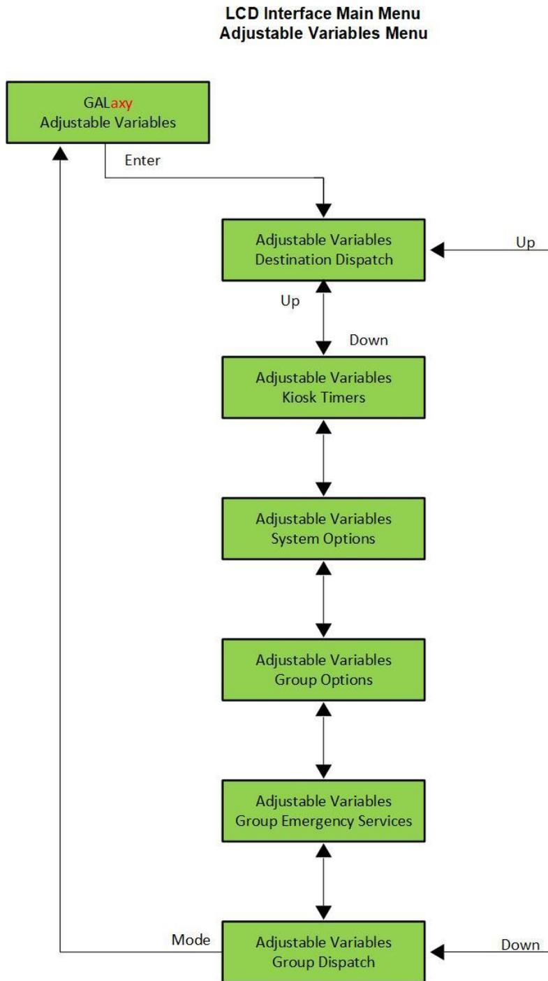
Figure 5-7: The Adjustable Variables Menu of the LCD Interface
