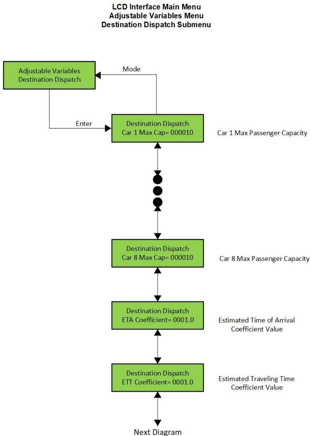
Figure 5-8-1: The Destination Dispatch Submenu of the LCD Interface
