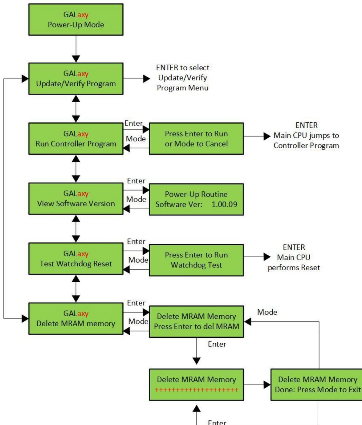
**Figure 5-18: LCD Interface Main Menu – Power-Up Mode Submenu**
