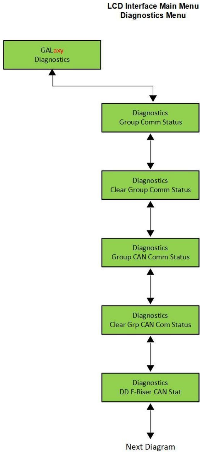
**Figure 5-3-1: LCD Interface Main Menu - Diagnostics**
