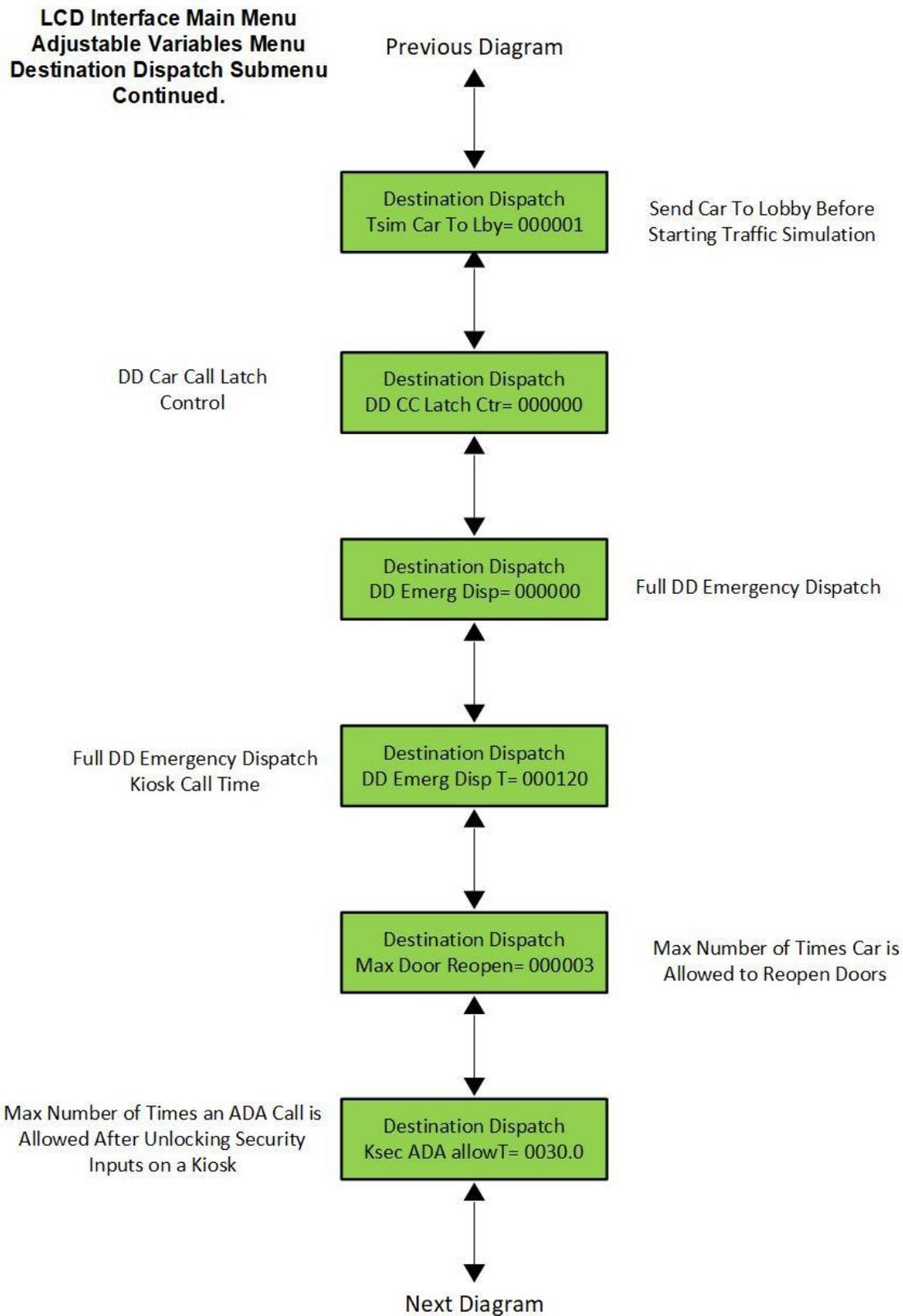
Figure 5-8-4: The Destination Dispatch Submenu of the LCD Interface
