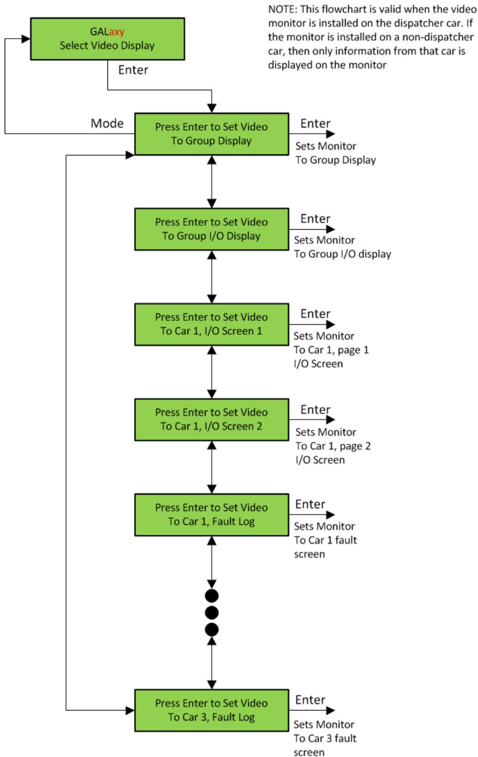
**Figure 5-22: LCD Interface Main Menu – Select Video Display**
