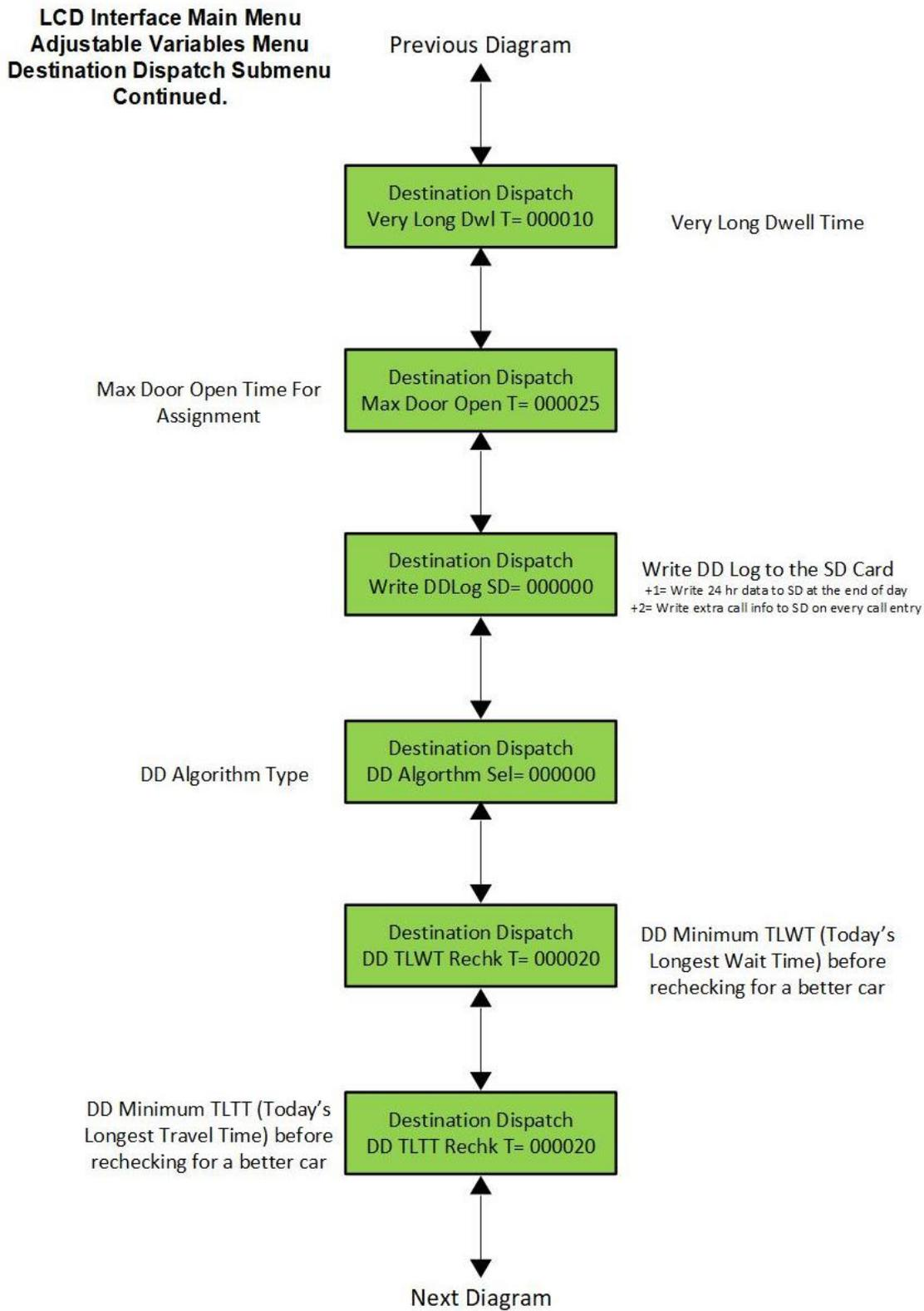
**Figure 5-8-2: The Destination Dispatch Submenu of the LCD Interface**
