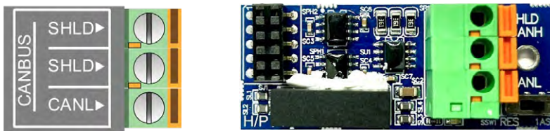
Figure 14: CANBUS wire terminals (left) and module, MOVFE-0009N (right).
